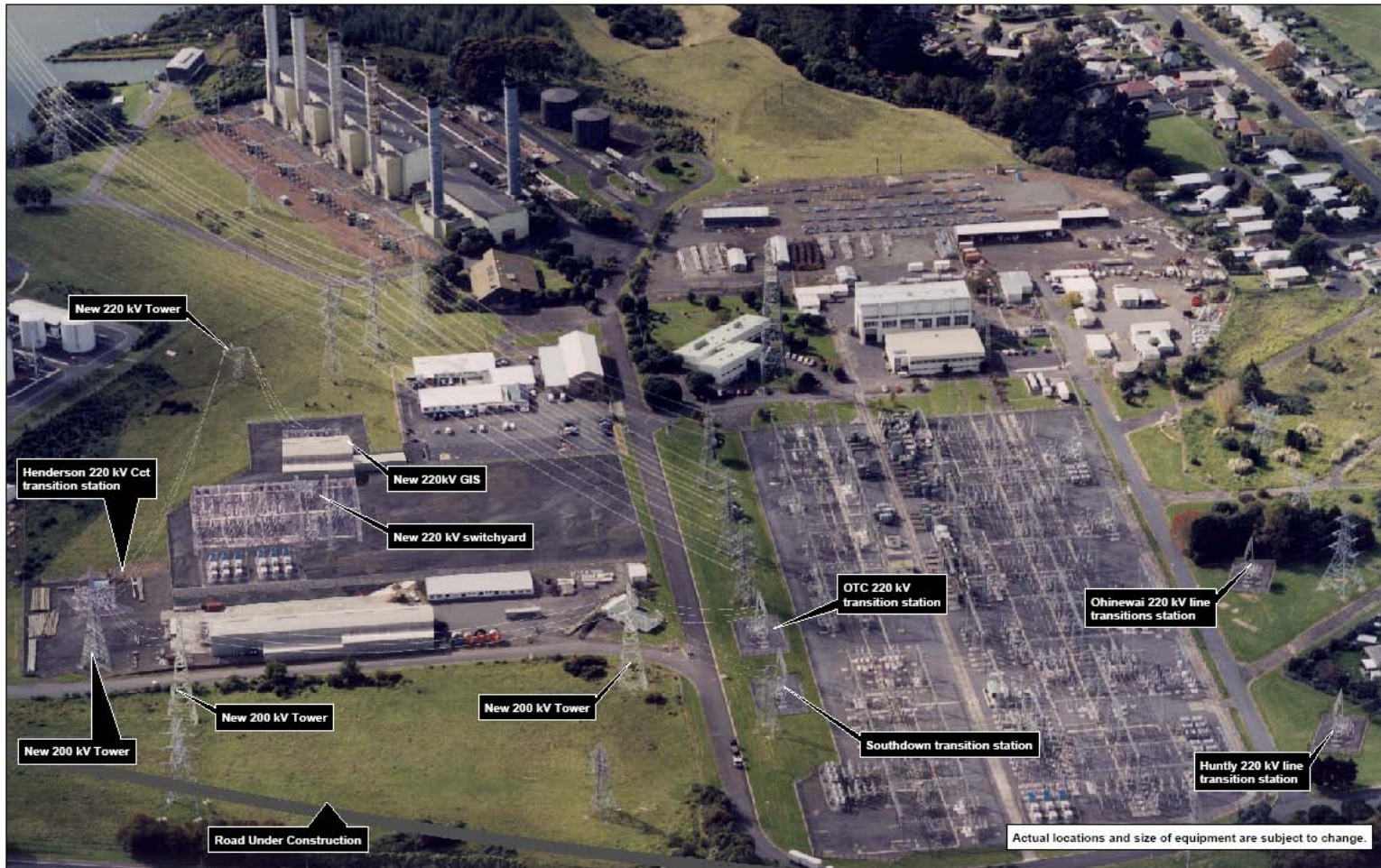
Indicative Proposed Otahuhu 220 kV GIS Layout July 2007
