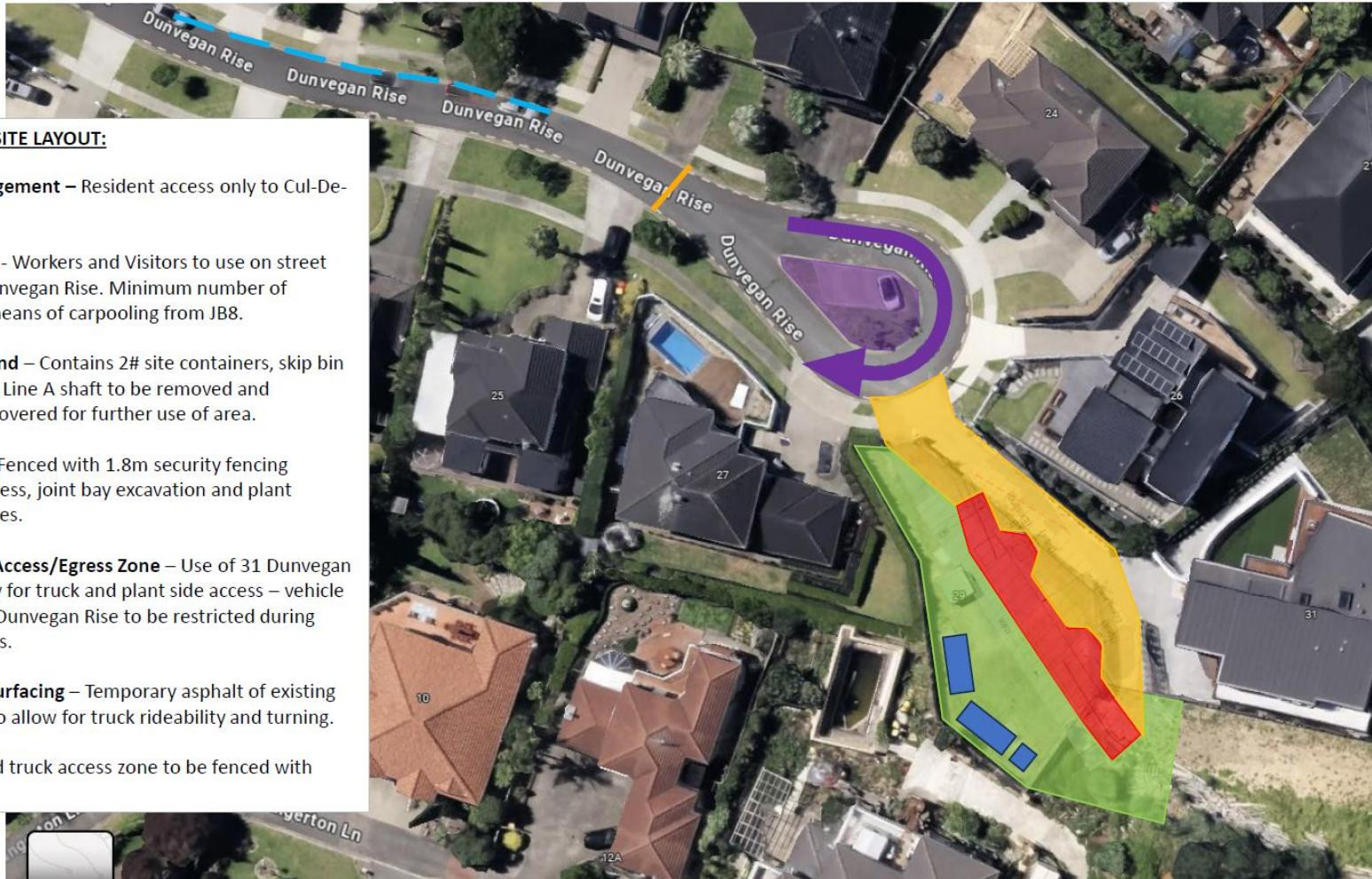
Entire works, compound and truck access zone to be fenced with 1.8m high security fencing.
