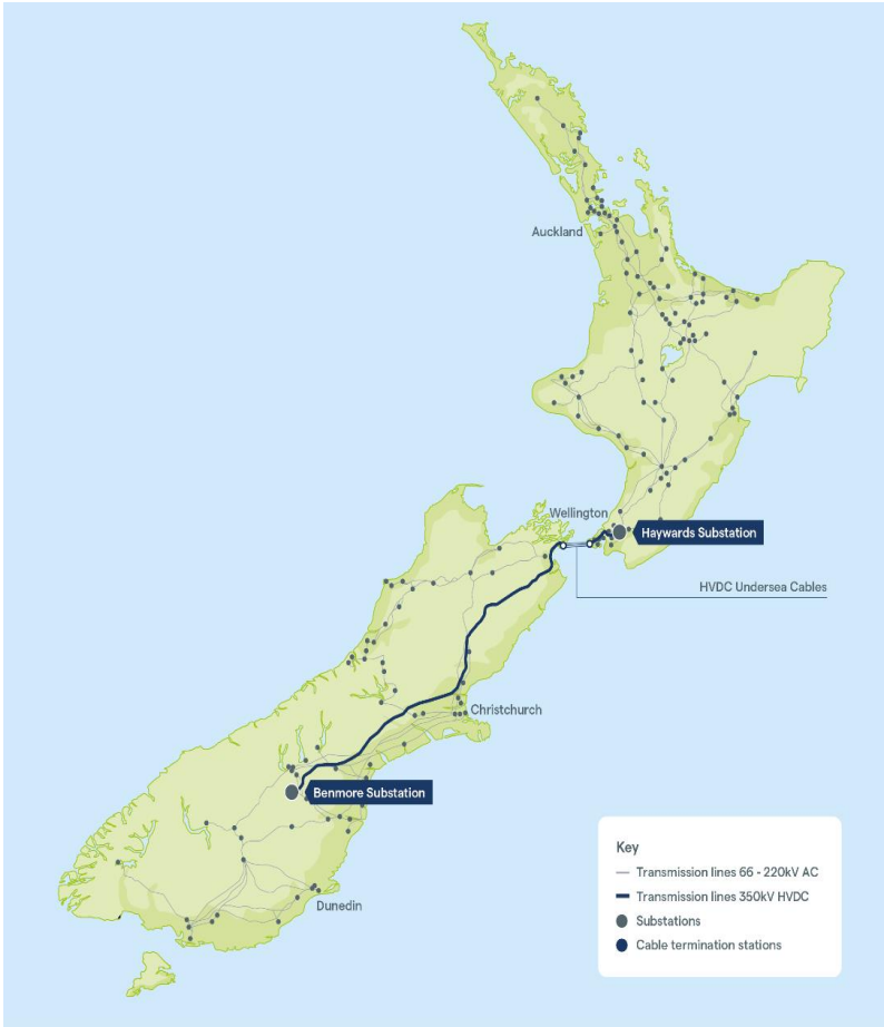
Figure 1: Overview of the New Zealand Transmission Network showing the HVDC link
