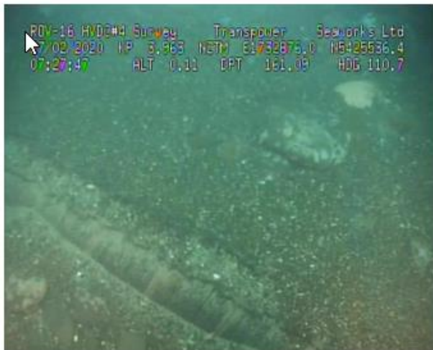
Figure 4: Serving damage - wide pattern KP3.963
