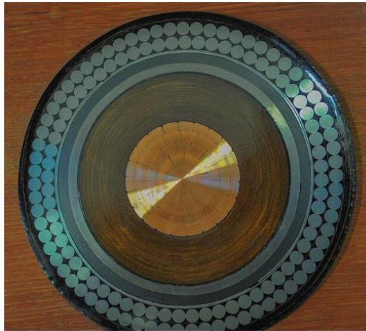
Figure 1: HVDC Submarine cable Cross-section (key stone conductor), 127mm Outside Diameter.
