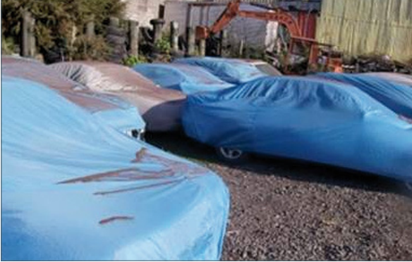
Vehicles covered to avoid fouling from tower cleaning discharges.
