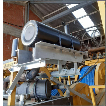
New muffler on a conductor wiring machine to mitigate noise when used in urban areas.
