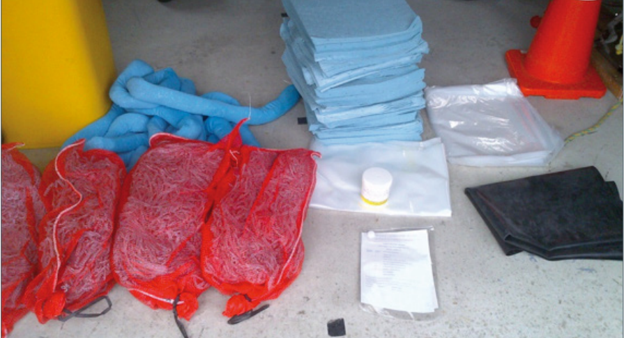
Contents of Transpower supplied wheelie bin oil spill kit deployed at all substations. Use of its contents is described in Section 18.
