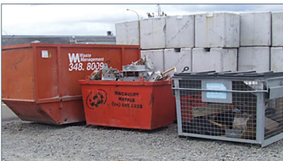
Segregation of general waste, scrap metal, Paper and Cardboard at a depot. This depot also recycles aluminium and insulators (which are crushed, the metal being recycled and the porcelain/glass used in sealing roads)
